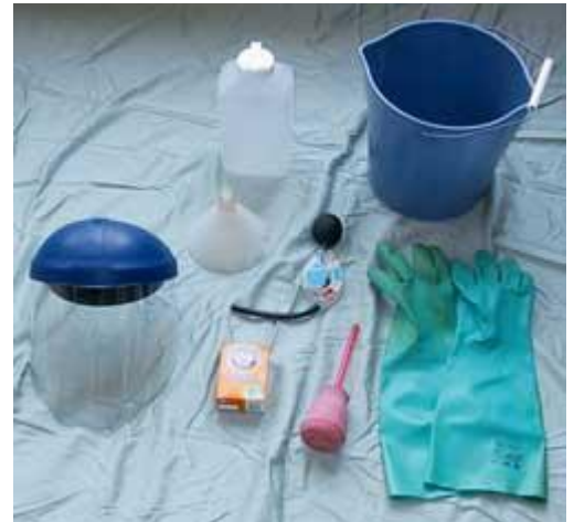
Required battery maintenance tools
